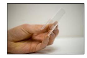
D 263® T eco is a colorless, low auto-fluorescence borosilicate glass with excellent transmission in the UV to NIR range, is lightweight,
