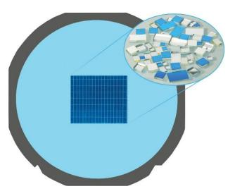
tolerances such as 0.025 mm with consistent perpendicularity of edges to faces is needed. Camera assist can also use fiduciaries, notches, flats, and matched corners as the precision locating feature. This process is key when small optical components must be fit/press fit, or hermetically sealed and in need of low cosmetic, chip free defects and a near "100%" coated clear aperture for imaging, sensing, laser beam steering, indicators, and sighting.
