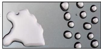
fingerprints wipe off easily and the coating provides a non-smudge Surface. The hydrophobic properties repel water and other liquids, allowing for them to be shed easily from the glass, promoting easier "view-ability". CleanVue™ PRO's hydrophobic coating properties also reduce friction on the glass, providing improved surface "slickness", enhancing scratch resistance.
