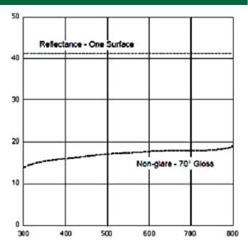
The lower the gloss units, the less glare. Abrisa Technologies can provide non-glare or anti-glare soda lime glass with the following gloss unit specifications:
