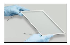
Utilizing ultrasonic soldering makes it possible to apply bus bars and lead wires in a single step, directly to the glass or ITO conductive surface, rather than using a more costly multi-step conventional etch and print process.
