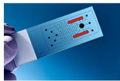
EN-A1 is ideal for these applications due to its high transmittance (400 - 2300 nm), its good chemical resistance, its coefficient of thermal expansion (CTE of  $38 \times 10^{-7}$ ), and its low fluorescence at genomic excitation wavelengths. EN-A1 is available in sheet sizes of up to  $25'' \times 20''$  and can be ordered in standard thicknesses of 0.3, 0.5 and 0.7mm.
