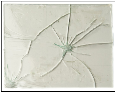
Chemically Strengthened Glass Break Pattern
