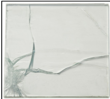
Non-Tempered/Strengthened Break Pattern
