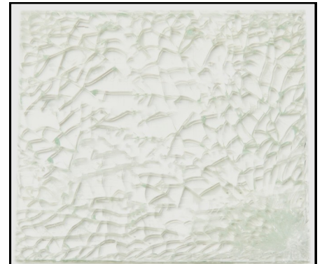
Heat Tempered Break Pattern
